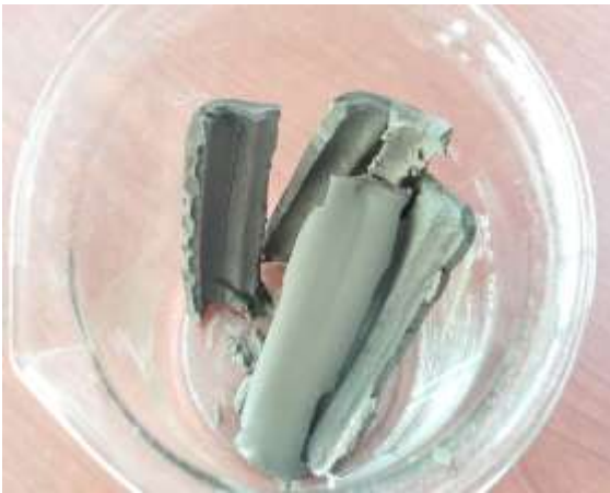
Fig. 3 Cake and particle morphology of BaSO 4 precipitates after candle filtration
